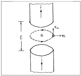
Figure 2. The arc as an MHD generator.
