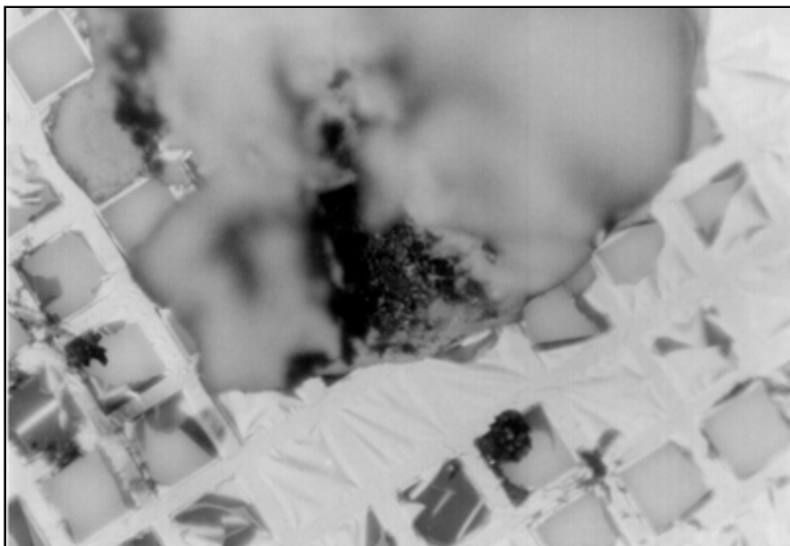
Transmission Electron Microscope grid on which the copper-containing flake (dark piece in center) is mounted on solidified correction fluid (large gray area). Photo courtesy: Cincinnati Group
