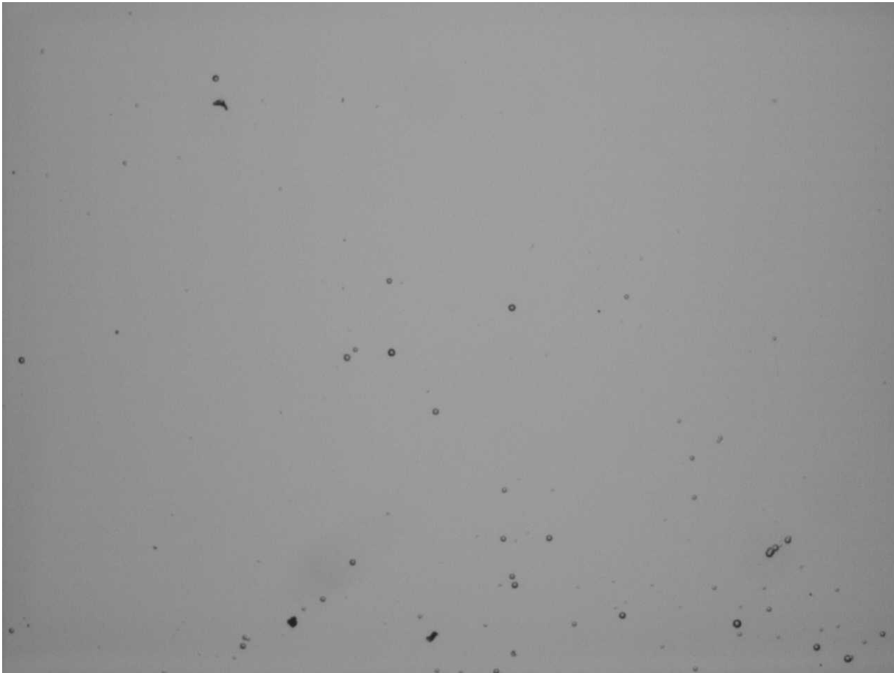
Figure 4 A small cluster of tracks. Magnification 40. The photographed area is about 1.3 mm by 1.0 mm. This figure shows what is above Figure 3.
