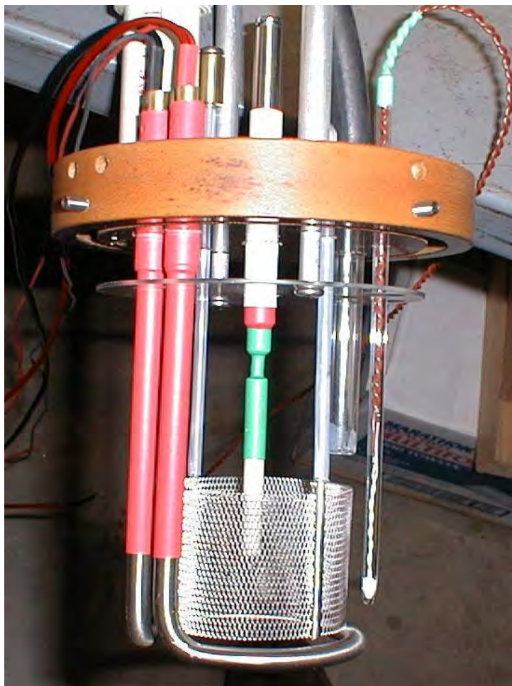
Figure 3 Electrodes and other components mounted on the lid. The ring below the anode is the ohmic heater, the vertical glass tube on the right contains the thermistor. The transparent antispashing baffle can be seen below the lid. The side screws were used to mount the lid rigidly on our polycarbonate cell (note the deep groove on the lower surface of the lid). The tip of the tungsten cathode is shown in Figure 4 below.
