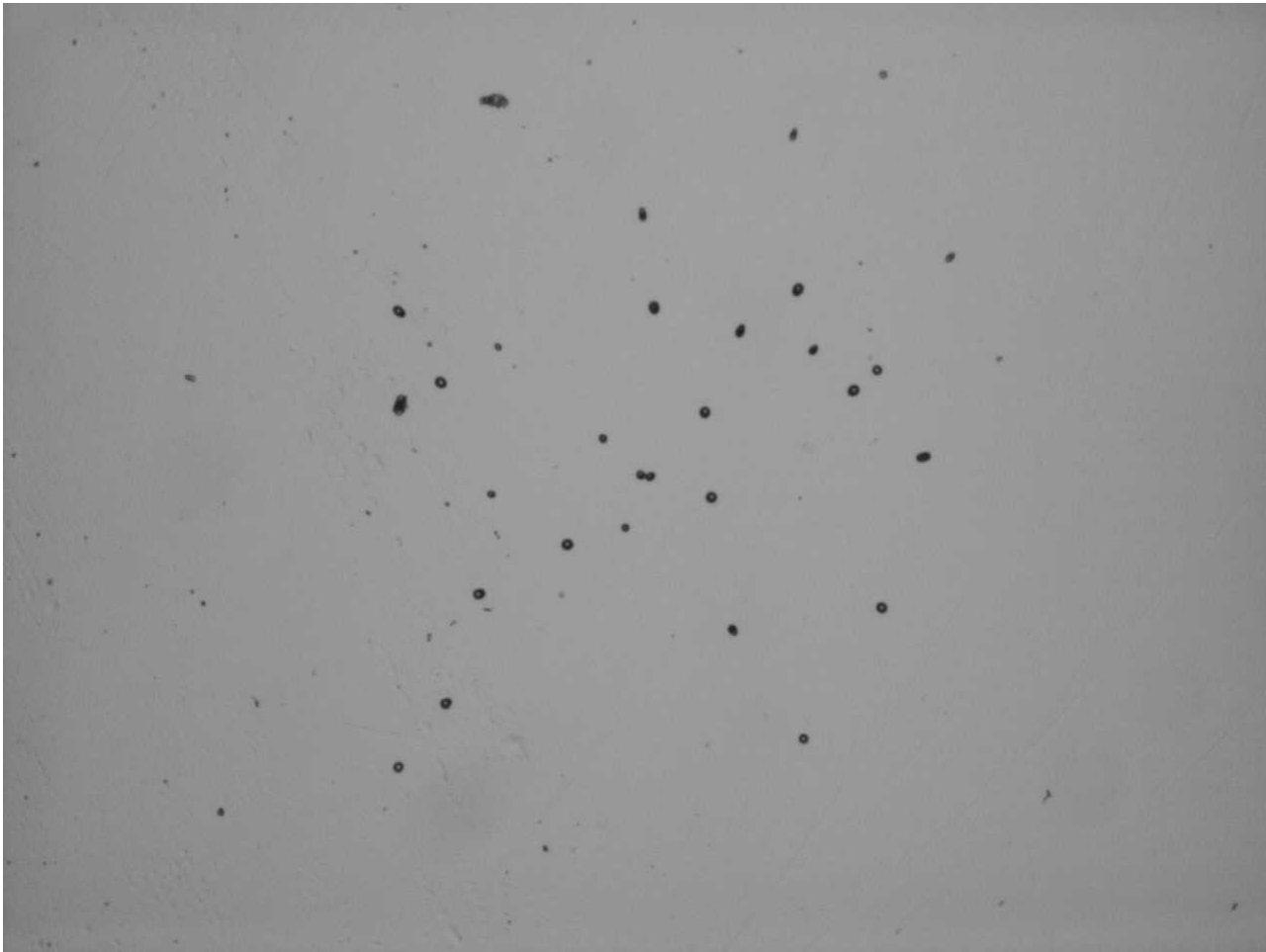
Figure 1 A small cluster of tracks. Magnification 40. The photographed area is about 1.3 mm by 1.0 mm =====
