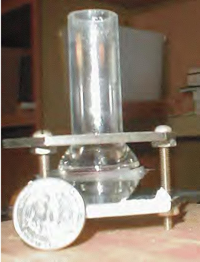
Figure 3 Cell #1. Two O-rings and the 6 micron mylar film (received from Oriani) are located between two parts made from glass. Cell #2 is not shown because it is just a polyethylene storage bottle with a removed lower part, as described above. The coin leaning on the cell has the diameter of 25mm. Let me add that glass components of Oriani cell can be ordered from: http://www.kimble-kontes.com/html/pg-671750.html The inner diameter of tubes are close to 16 mm. -----
