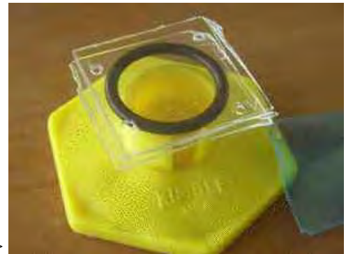
Figure 3 (A) Two flexible Viton o-rings are pressed against the CR-39 chip (by clamps applied to glass tubes) to prevent leakage of the electrolyte. The inner diameter of each tube was close to 15 mm; the wire diameters (Pt and Ni) were 0.5 mm. The Ni cathode was a “foot” supporting the rigid anode-cathode structure. (B) A CR-39 chip on top of an o-ring, as used to detect nuclear particles emitted after electrolysis.
