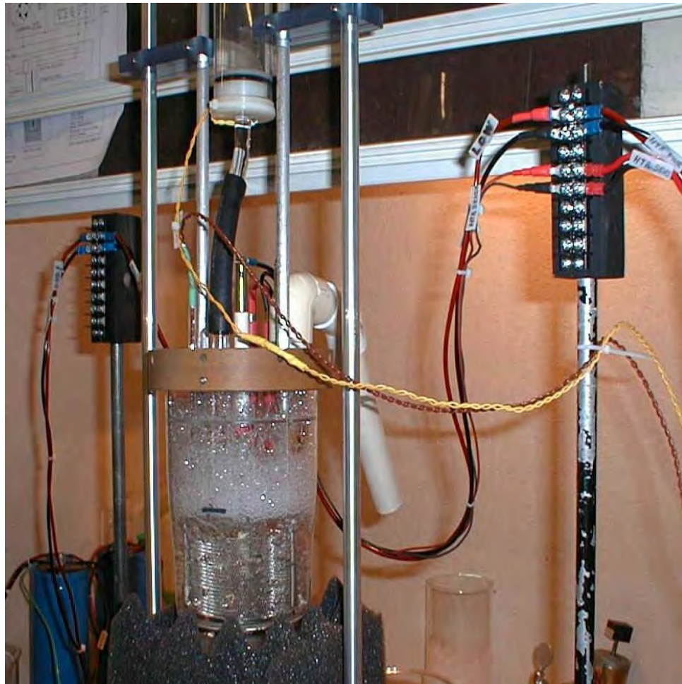
Figure 2 The photo of the setup showing the foam above the electrolyte. The dark cushion below the vessel helped to prevent bouncing of the scale. The inner diameter of the white PVC pipe was about 22 mm.
