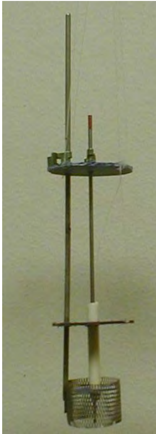
Figure 1 The cathode (shorter tungsten rod) and the anode (welded to the longer Ti rod), suspended by a nylon thread, are being lowered into the beaker. Rigidity was assured by two plastic disks (sterilite remains rigid at 100 C). The second function of the lower disk was to act as an antispashing baffle, inside the electrolyte.
