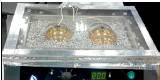
Sample sphere at left (84.1°C), control sphere right (79.6°C), aluminum bed of beads (80.0°C).
